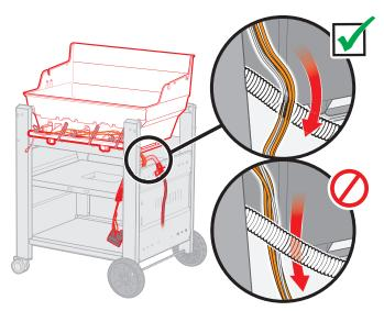
Route wires to the outside of the corrugated gas line.
