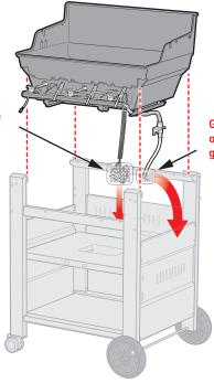
Gas line must be routed on the <u>OUTSIDE</u> of the grill frame.
